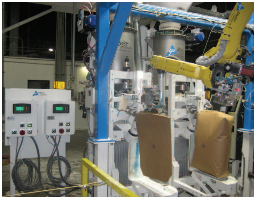
The robotic arm (yellow) automatically places empty paper valve bags on the air packers' fill spouts, reducing the operation's need for manual labor.
